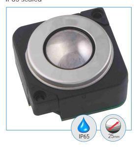
The GS25 series are ruggedised professional trackballs. The ball and the trim are made of quality stainless steel. The double-sided seal ring provides sealing to IP65 static (ball in rest). Stainless steel shafts and bearings ensure a solid and precise pointer control. The unit has been designed to be back of panel mounted as part of OEM keyboards and consoles. The GS25 is an ideal pointing device for applications with restricted mounting space.
