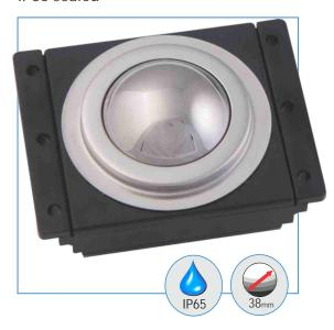
The GS38 series are ruggedised professional trackballs for vandalproof applications. The ball and the trim are made of quality stainless steel. The double-sided seal ring provides a sealing to IP65 static (ball in rest). Stainless steel shafts and bearings ensure a solid and precise pointer control. The unit can be used for frontpanel mounting (remove the mounting bracket) or for backpanel mounting.
