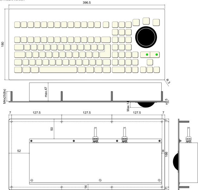
COLOURS Metal enclosure : RAL7037 Dusty grey Keyboard background : RAL7035 Light grey Key edges : RAL7037 Dusty grey Key legends : RAL9005 Jet Black Dim in mm.
