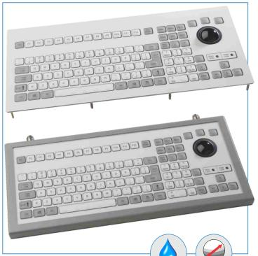
The unit features a full MF (multi-functional) keyboard with separate numeric-, cursor- and control keypads. The robust industrial grade trackball has a ball diameter of 38 mm and allows highest precision in cursor control. The keyboard part is sealed to IP65, the self-adjusting PTFE seal of the trackball enables an IP65 static (ball in rest) protection grade. Colour scheme and legend styling fit with the most recent industrial computer equipment.
