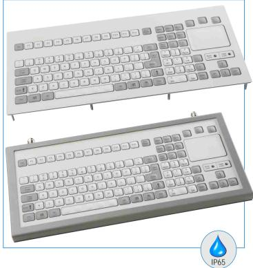
The unit features a full MF (multi-functional) keyboard with separate numeric-, cursor- and control keypads. The touchpad uses the Field Distortion Technology to sense the presence of your finger. This device is not pressure sensitive, a light touch is sufficient, tracking your fingertip precisely. The complete unit is sealed IP65. Colour scheme and legend styling fit in with most recent industrial computer equipment.
