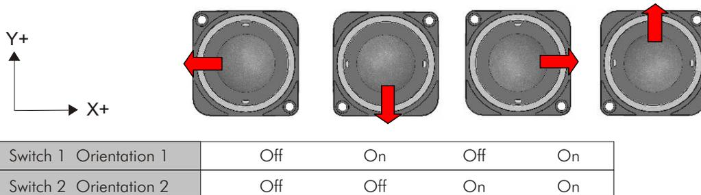
Figure.1 Mounting Orientations
