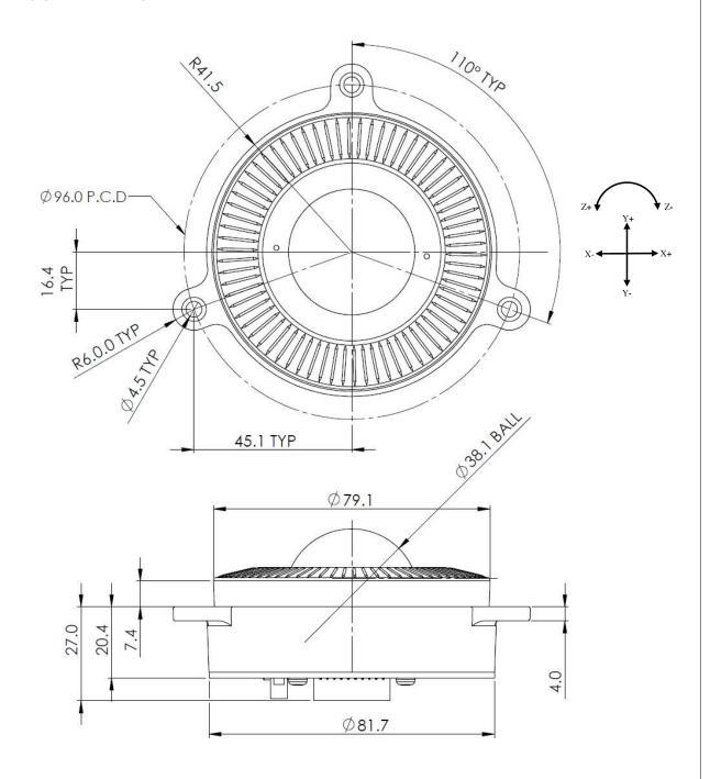
Dimensional drawing specifies factory default orientation. All dimensions are in mm unless otherwise stated.
